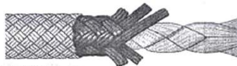
Figure 5 Plaited core braid rope and, in the picture above, (right).
