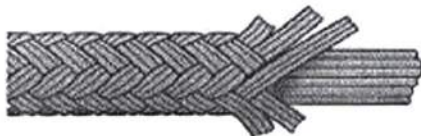
Figure 3 Parallel core braid rope and photographic example below.
