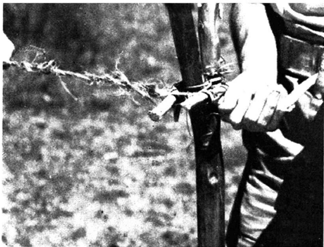
Bark fibre being spun into strands using a single crank handle.
